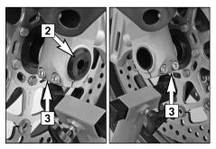
Loosen the collar screw [2] and the clamping screws [3] on both fork leg axle passages. Unscrew the collar screw approx 8 turns, press on the collar screw with your hand to push the wheel spindle out of the fork leg axle passage and remove the collar screw. Hold the front wheel while you pull out the wheel spindle.
