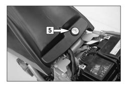
Remove the seat and screw [5]. Close the fuel taps and fuel line. Slightly pull the tank towards the back, lift about 10 cm (4 in) in the front and slide it under the tank a little bit to hold it in this position.
