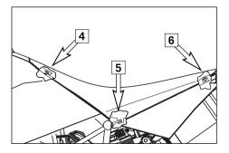
To mount the seat, attach the seat to the oval head screw [4], lower the seat in the back while sliding it towards the front. Both noses [5] should fit into the frame. Insert the catch bolts [6] in the lock housing and push the seat down in the back until you hear the catch bolts snap into place.
